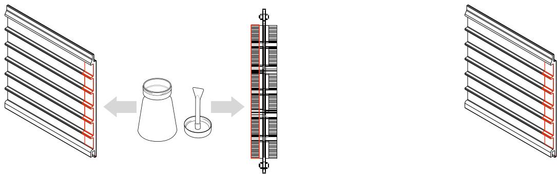
Min. distance 20 mm / max. distance 50 mm
